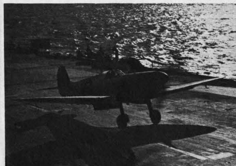
SEAFIRE Familiar elliptical wing stands out in shadow cast on the flight deck by a Seafire II taking off from H.M.S. Illustrious. An adaptation of the Spitfire V, this Seafire does not have the
